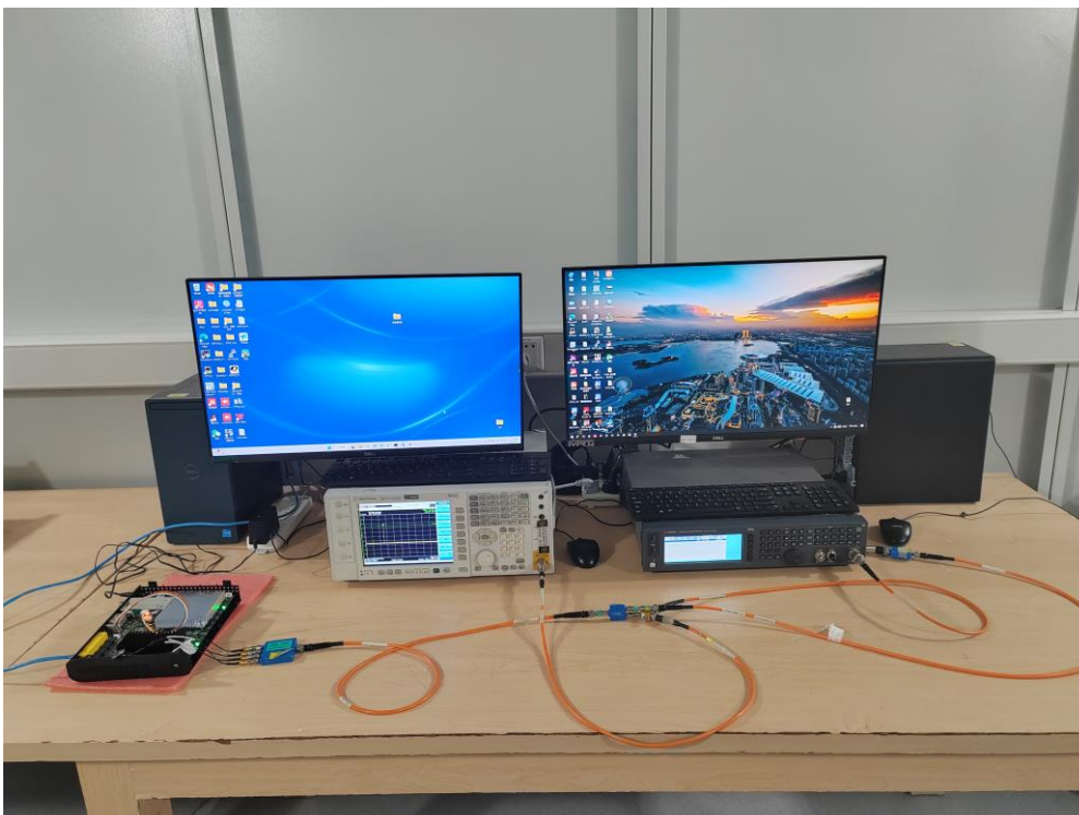
Description: DFS Test Setup
