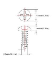
Figure 2: Recommended Screw Size
