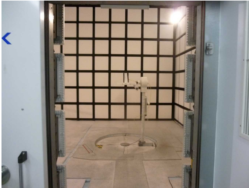
Photo 1: EUT at the anechoic chamber
