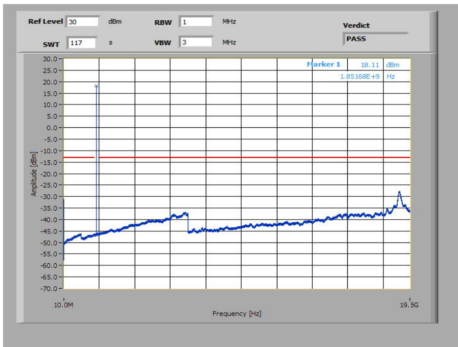
Plot 4: 3 MHz – QPSK - Lowest Channel (10 MHz – 19.5 GHz)
