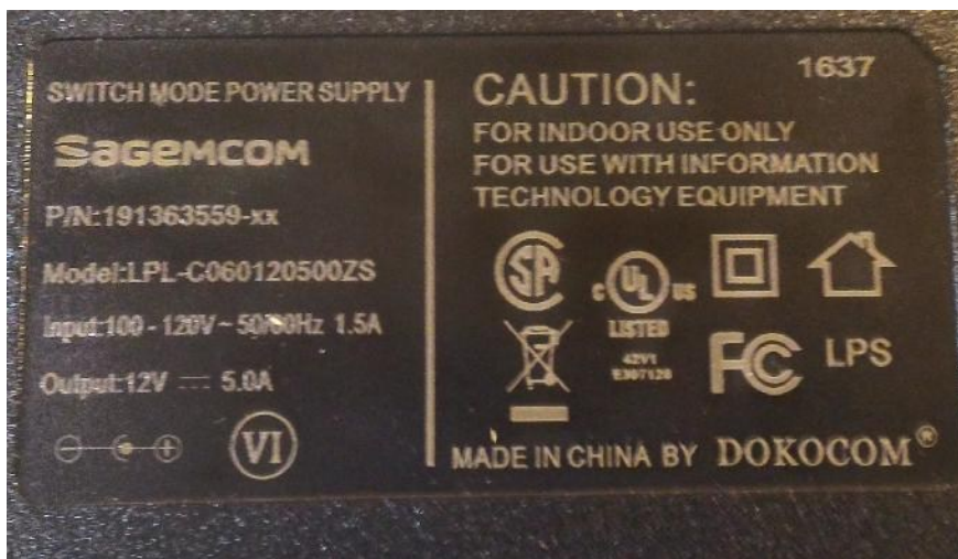
Power supply n° 2
