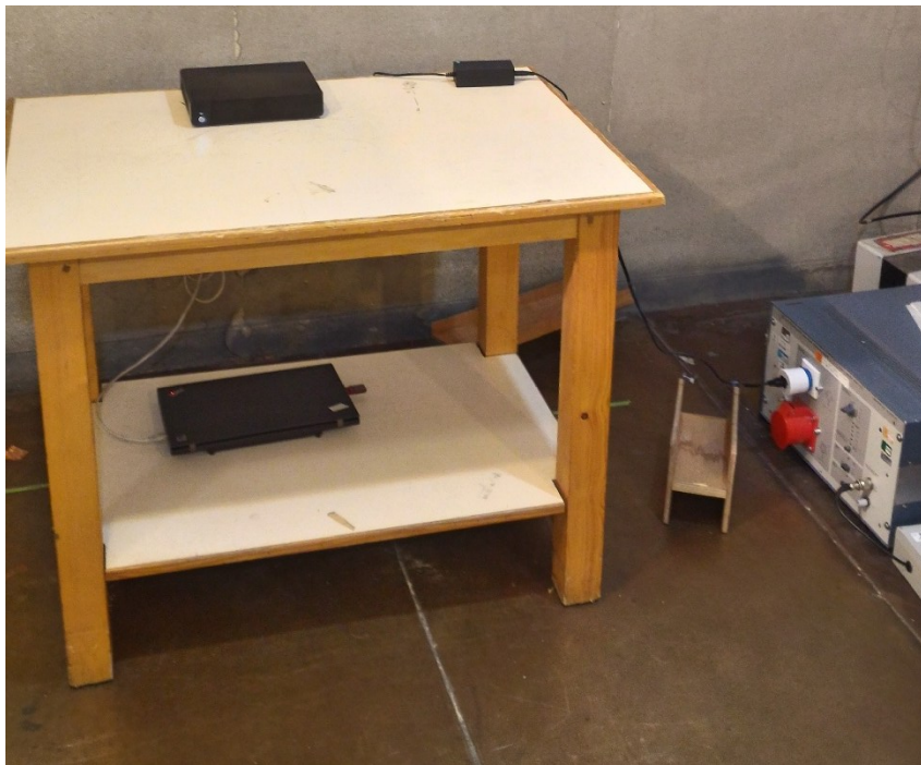
Photograph for AC Power Line Conducted Emissions (Front view)
