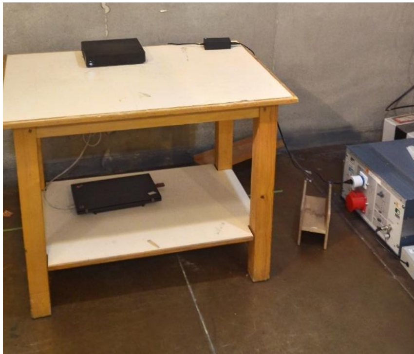
Photograph for AC Power Line Conducted Emissions (Front view)
