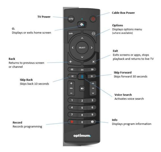
There is no need to point the remote directly at the box in order to control it. You can aim your remote anywhere. You must pair the remote to your TV in order to work the TV power, volume and mute controls.
