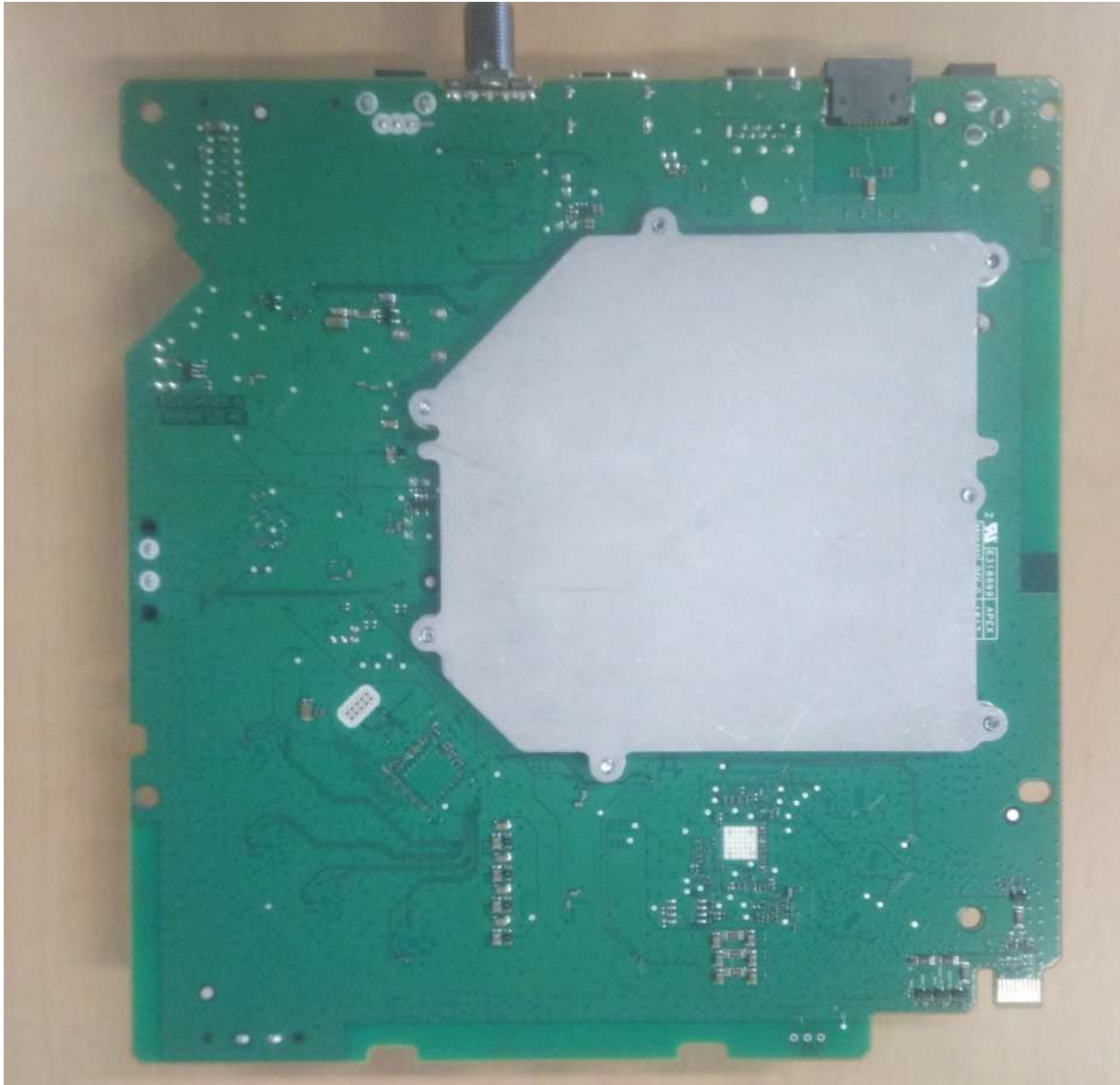
Main Board face 2 with Shielding
