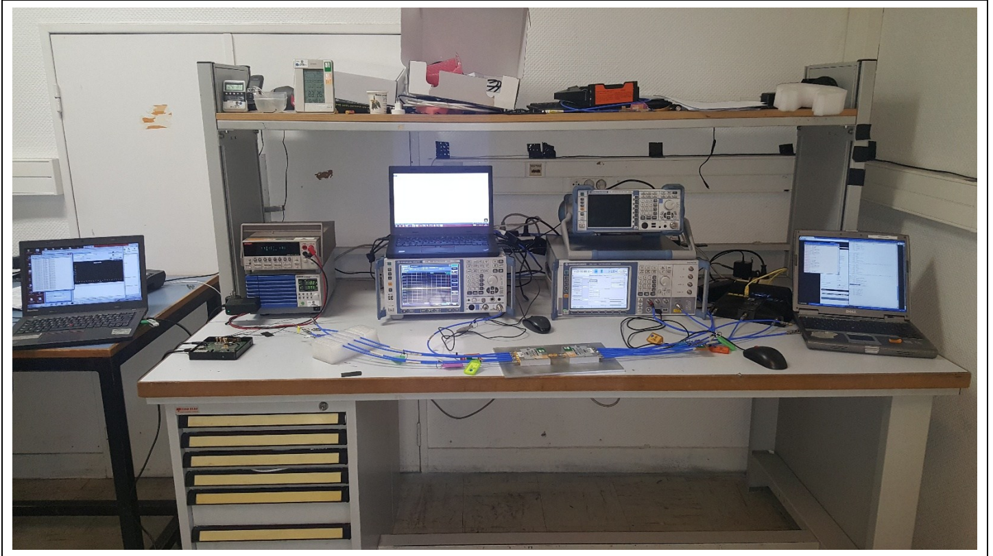
Photograph for DFS Non-Occupancy Period
