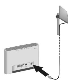
Screw the connector of the antenna cable into the ANT WIMAX connector on your SX682 WiMAX. In order to disconnect the antenna cable from the connector, open the screw connection. I
