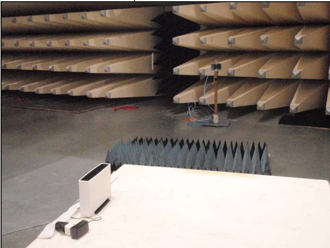
Photo 4: setup of radiated emission > 1 GHz
