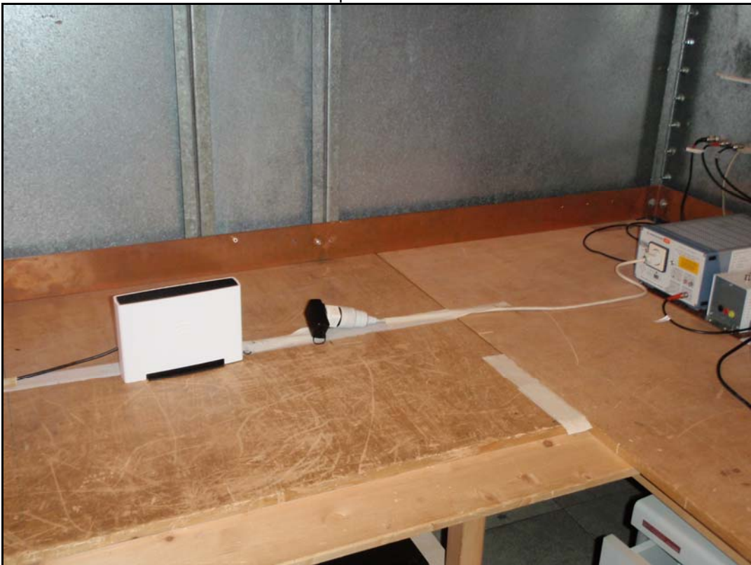
Photo 6: s setup of conducted emission
