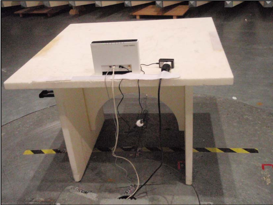
Photo 2: setup of radiated emission
