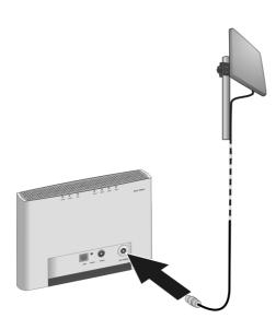
Screw the connector of the antenna cable into the ANT WiMAX connector on your SE681 WiMAX. In order to disconnect the antenna cable from the connector, open the screw connection.
