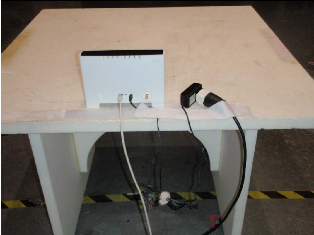
Photo 2: setup of radiated emission
