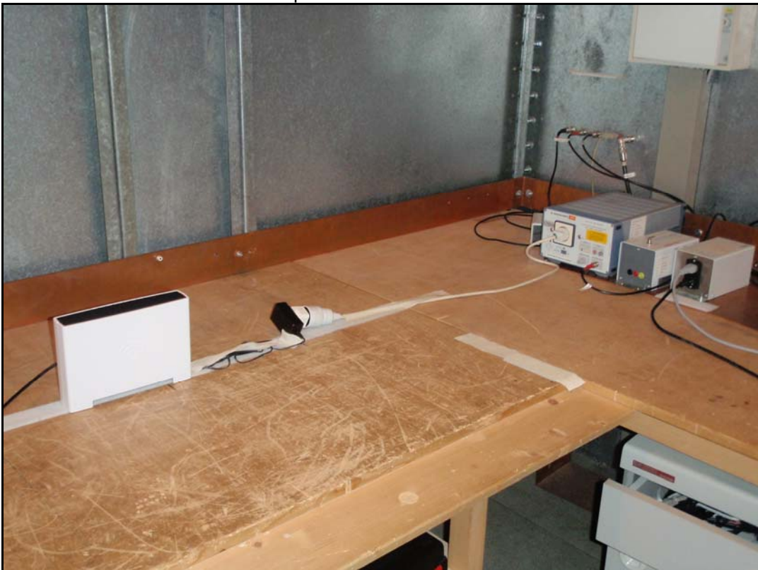
Photo 6: setup of conducted emission on mains
