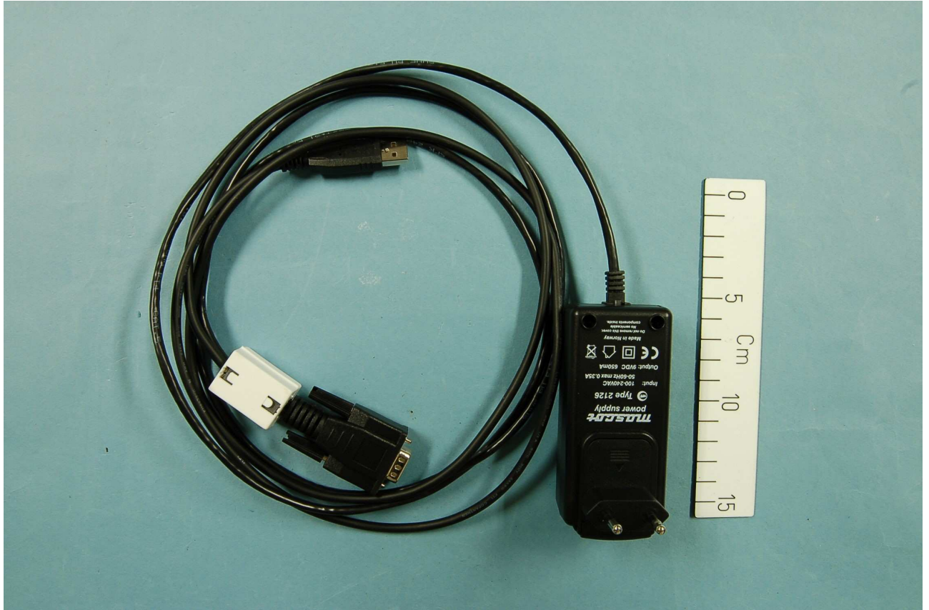
Charger with USB cable, Ferrite 28A2029-A0
