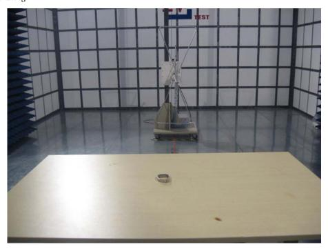
Radiation Emission Test Setup (Above 1GHz)
