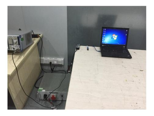
Radiation Emission Test Setup (Below 30MHz)
