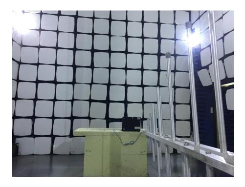
Radiation Emission Test Setup (Above 1GHz)
