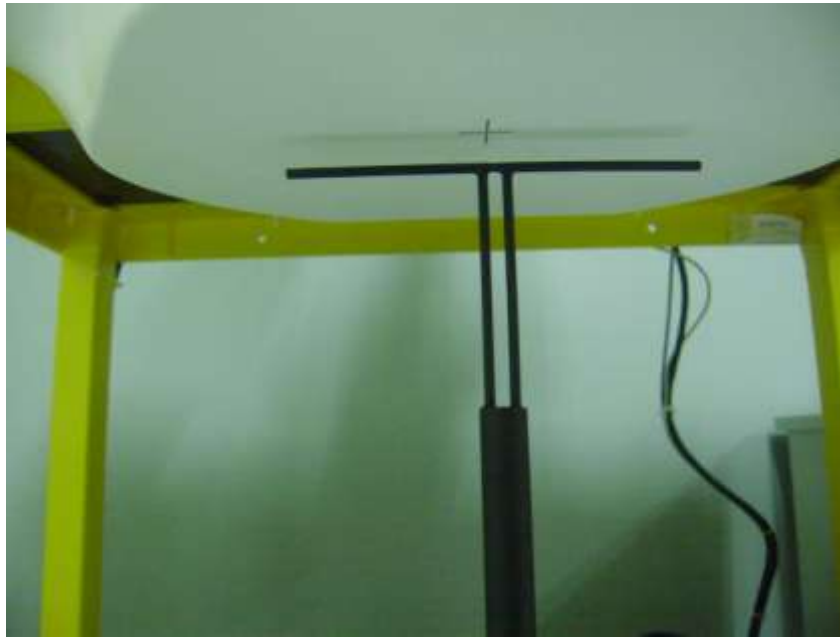
Fig 6.2 Setup Photo of Dipole Antenna
