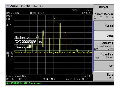
a slot of pulse=0.525ms,total pulse=10,T<sub>on</sub>=(0.525\*10)=5.25ms
