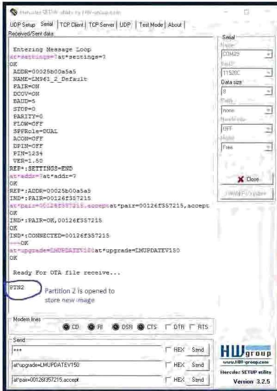
Figure 3. UART messages when the adapter opens a partition to write a new image
