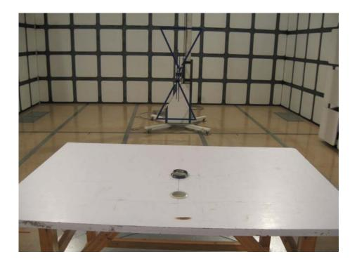
**Radiation Emission Test Setup (Above 1GHz)**
