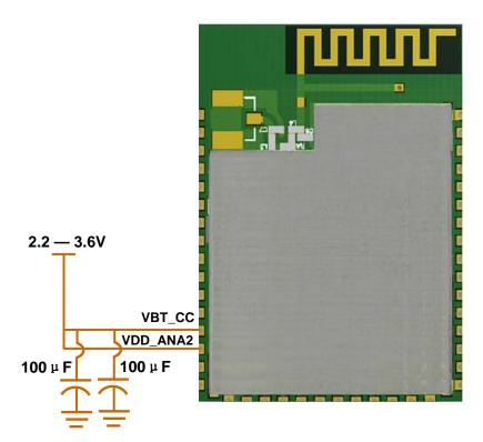
Noted: The device can draw up to 600mA for 25mS. Consider adding extra decoupling capacitors if the battery can not source the current. And please also make sure these two capacitors are closed to the port of VBT\_CC.
