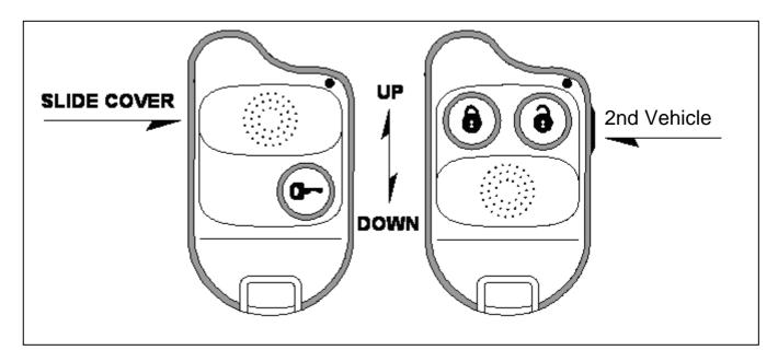
The slide cover is used to protect pressing buttons by accident. Move cover to middle position to block all 3 buttons.
