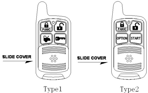
The slide cover is used to protect pressing buttons by accident. Move cover to up position to block all 4 buttons.
