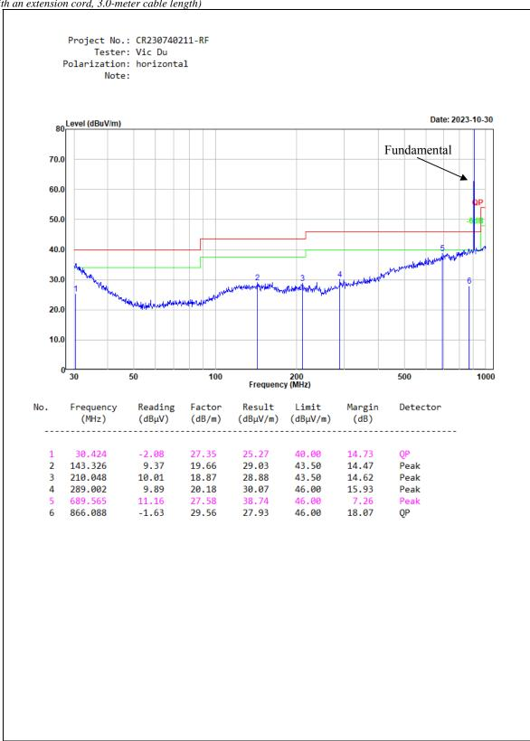
Test plots for maximum output power channel: low channel (EUT equips with the antenna which is mounted on a sucker with an extension cord, 5.0-meter cable length)
