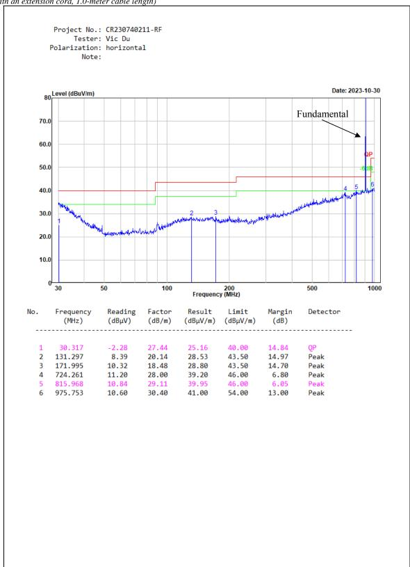
Test plots for maximum output power channel: low channel (EUT equips with the antenna which is mounted on a sucker with an extension cord, 3.0-meter cable length)
