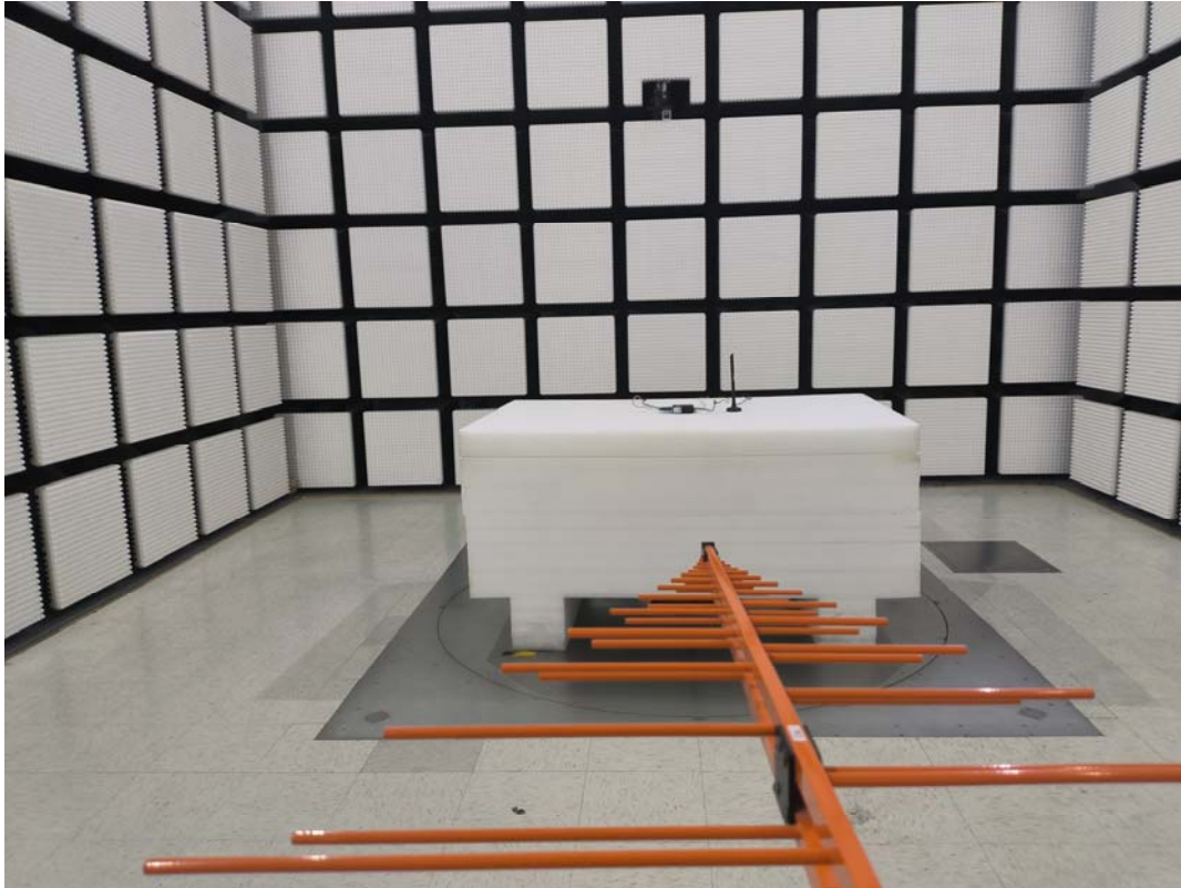
Radiated Emission Below 1GHz View (with antenna extension cable, 5m )
