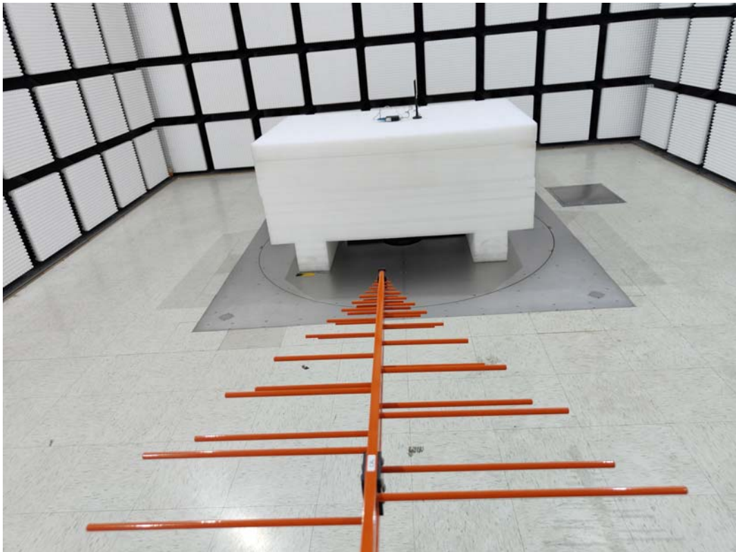
Radiated Emission Below 1GHz View (with antenna extension cable, 5m )
