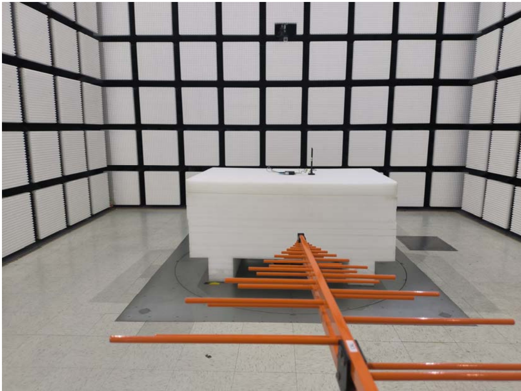
Radiated Emission Below 1GHz View (with antenna extension cable, 1m )
