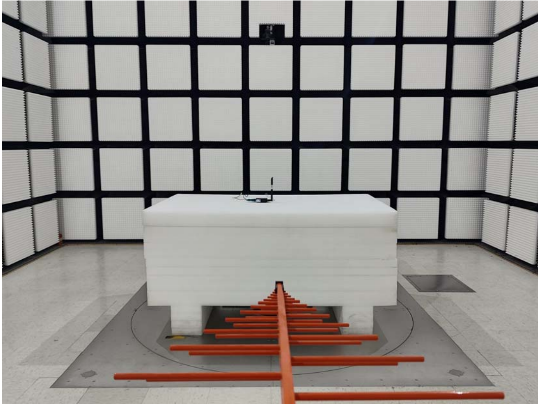
Radiated Emission Below 1GHz View (with antenna extension cable, 1m )
