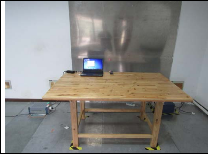
Conducted Emissions Test Setup Front View
