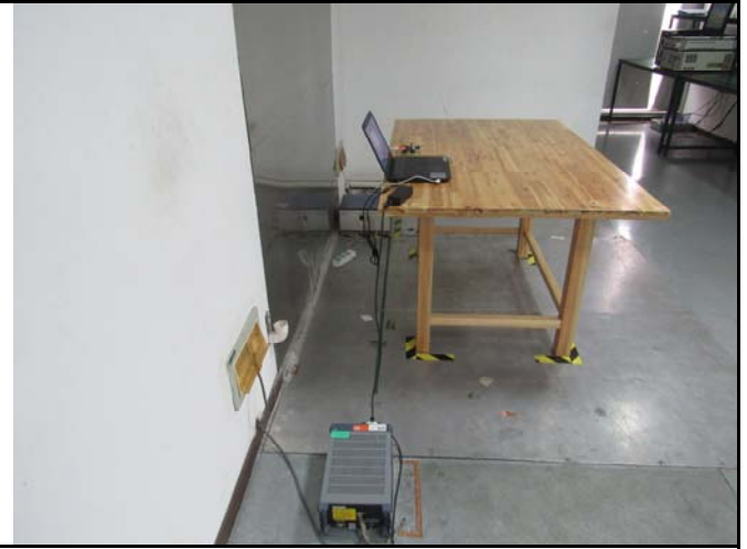
Conducted Emissions Test Setup Side View
