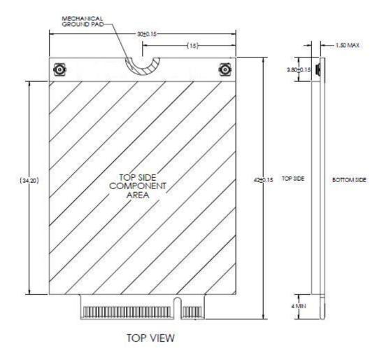
There are three connectors located on N5321 card: two RF connectors located in the top corners and one system connector located on the lower edge.
