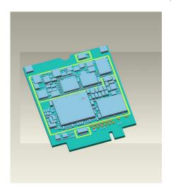
All major components are covered by EMC shields. All power and communication is routed through the edge connector of the card. The fastening hole in the upper corner is connected to ground.
