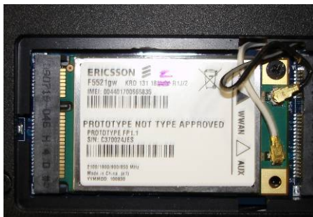
Figure A.2 The Ericsson F5521gw mobile broadband module.
