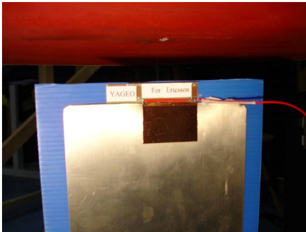
Figure B.1 Antenna #3 positioned with the top facing the ELI 4 phantom at 30 mm separation distance.
