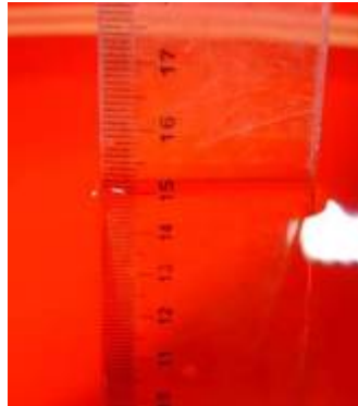
Measured level (152 mm) of 1900 MHz muscle tissue simulating liquid in the ELI-4 phantom
