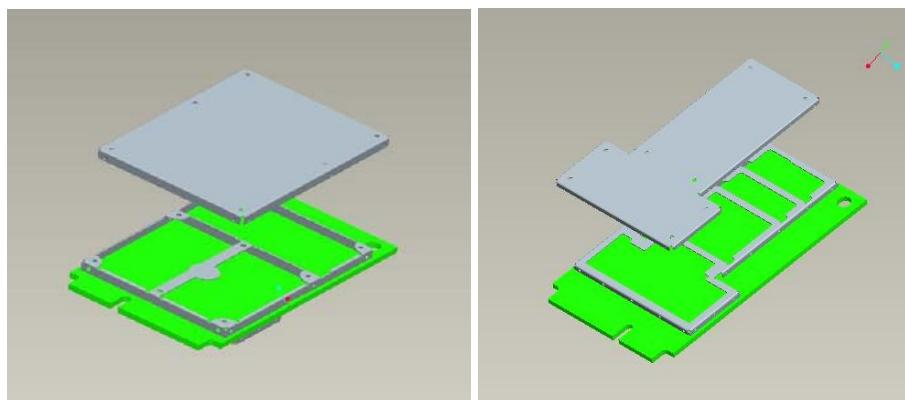
All components except the two antenna connectors are covered by EMC shields. All power and baseband communication is routed through the edge connector of the card. The fastening holes in the upper corners are connected to ground.
