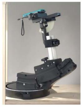
Fig. 10 Device holder supplied by SPEAG
