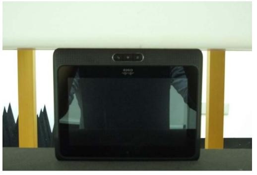
The EUT Secondary landscape is in contact to the ELI4 phantom distance is 0 mm.
