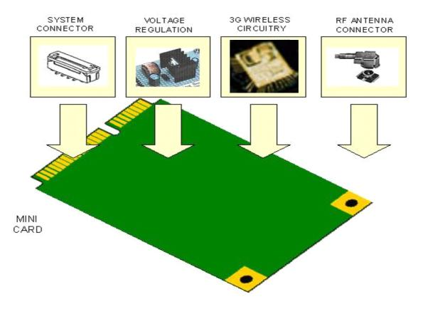
All components except the two antenna connectors are covered by EMC shields. All power and base band communication is routed through the edge connector of the card. The fastening holes in the upper corners are connected to ground.
