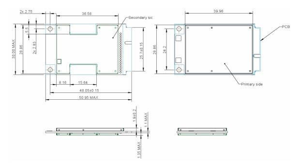
There are three connectors located on the card: two RF connectors located in the top corners and one system connector located on the lower edge, see the figure above.
