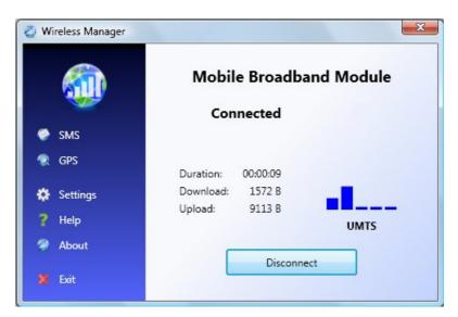
The network operator's and notebook manufacturer's logos can be customized in the application. Connection duration, connection mode, volume of data and an indication of the signal strength are provided in the Wireless Manager window while connection is active. Use the figures to provide an approximate checkpoint of the data volumes billed. Please note that the information shown here is not guaranteed to match the mobile operator's bill.
