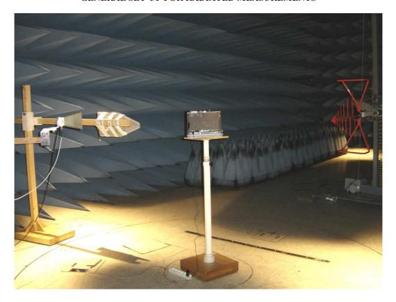
TEST SET-UP FOR RADIATED MEASUREMENTS BELOW 1 GHz
