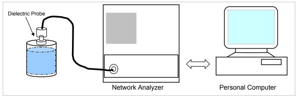
Set-up for liquid parameters check
