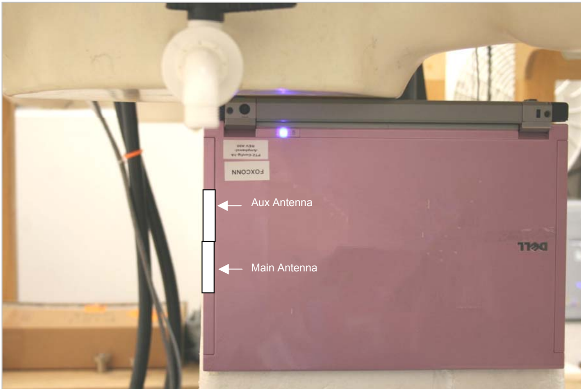
Setup Photo with Flat Phantom ELI4.0 (5 GHz Band)
