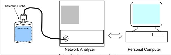
Set-up for liquid parameters check
