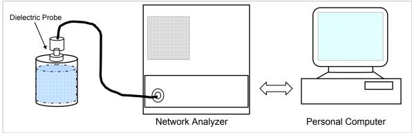
Set-up for liquid parameters check
