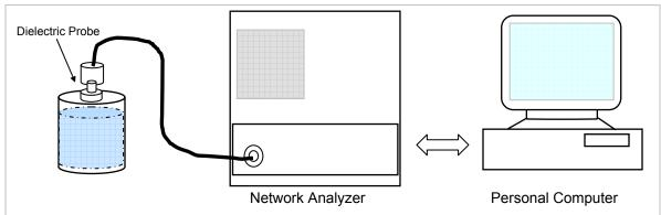
Set-up for liquid parameters check
