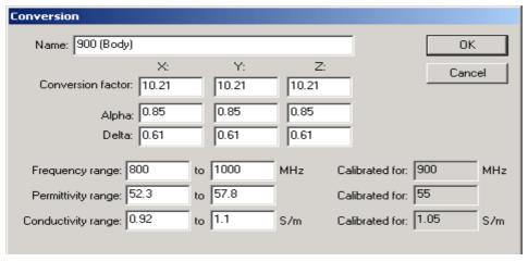
The measurement within the required frequency interval satisfy an expanded probe calibration uncertainty (k=2) <= 15% for all measurement conditions. Please refer to SAR report for probe and dipole calibration certificates produce by the system manufacturer.
