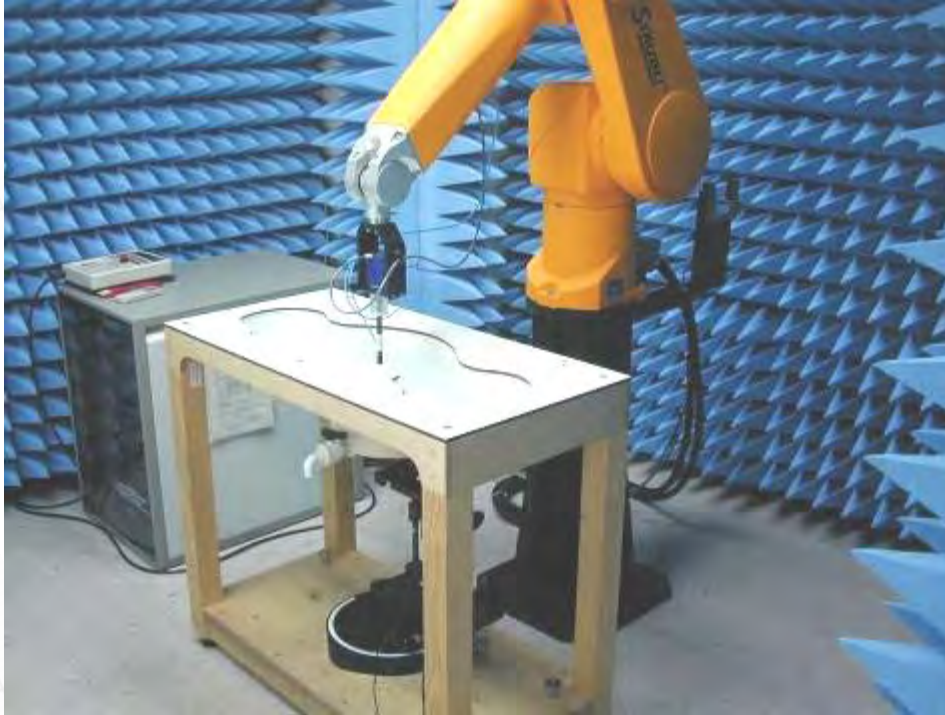
Fig.1 Photograph of the SAR measurement System
