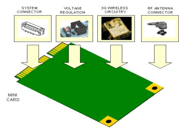
All components except the two antenna connectors are covered by EMC shields. All power and base band communication is routed through the edge connector of the card. The fastening holes in the upper corners are connected to ground.
