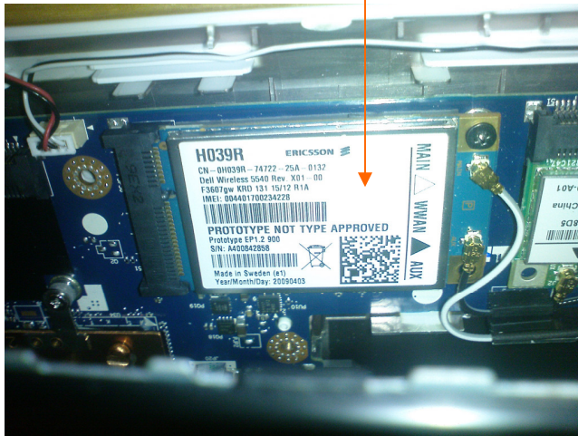
Figure A.2 Internal view showing the Ericsson F3607gw mobile broadband module.
