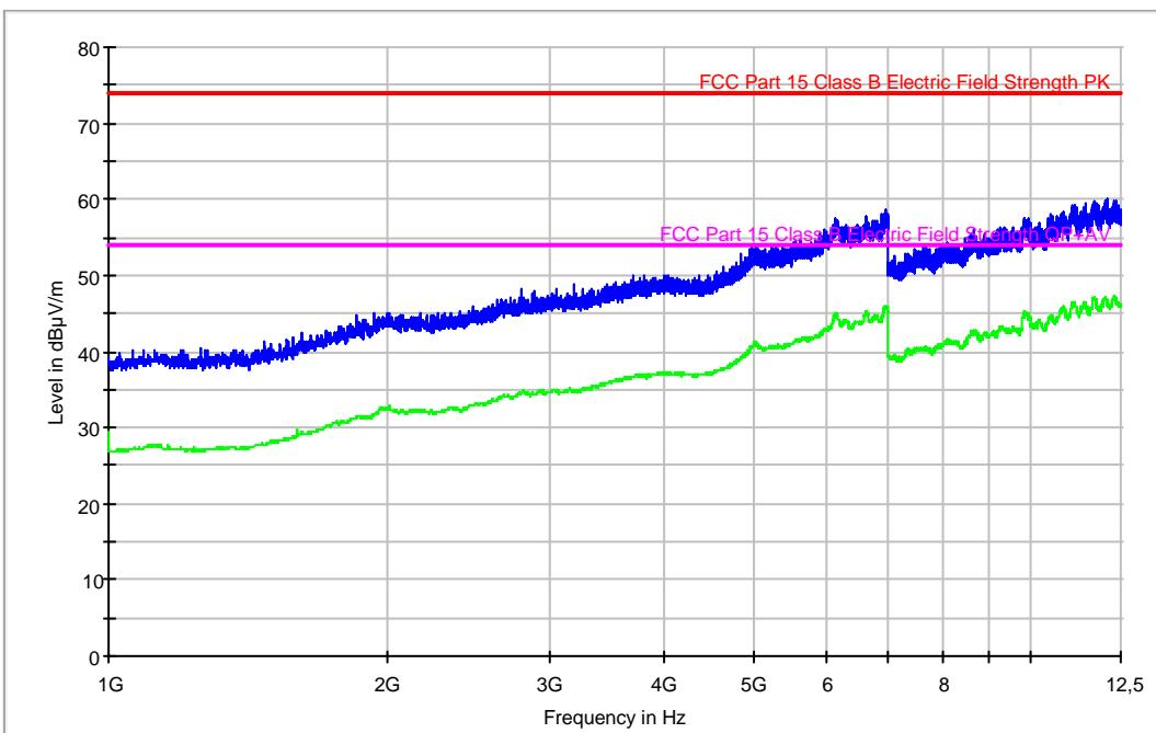
**Radiated Emission: CR0306 (1GHz to 12.5GHz Vertical polarisation)**
