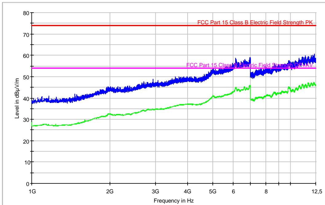
**Radiated Emission: CR0104 (1GHz to 12.5GHz Vertical polarisation)**
