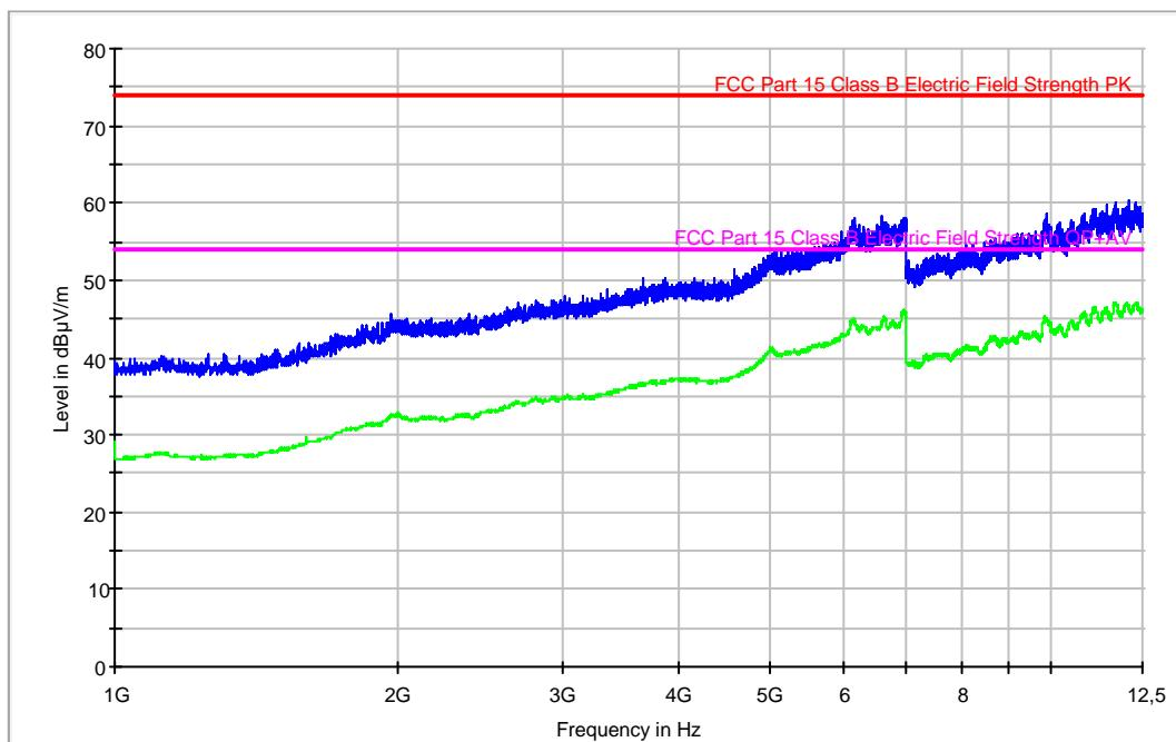
**Radiated Emission: CR0308 (1GHz to 12.5GHz Vertical polarisation)**
