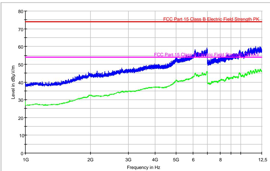
**Radiated Emission: CR0206 (1GHz to 12.5GHz Vertical polarisation)**
