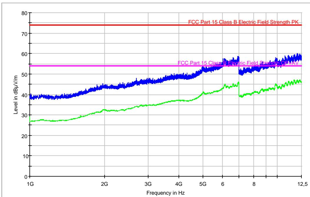
**Radiated Emission: CR0208 (1GHz to 12.5GHz Vertical polarisation)**
