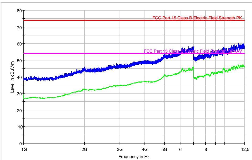
**Radiated Emission: CR0106 (1GHz to 12.5GHz Vertical polarisation)**
