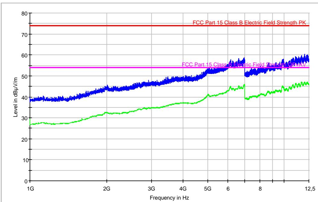
**Radiated Emission: CR0108 (1GHz to 12.5GHz Vertical polarisation)**
