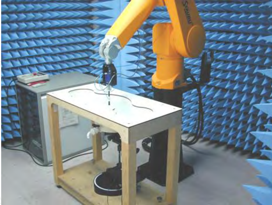
Fig.1 Photograph of the SAR measurement System
