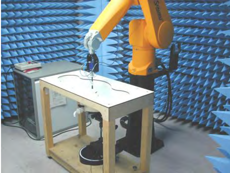
Fig.1 Photograph of the SAR measurement System
