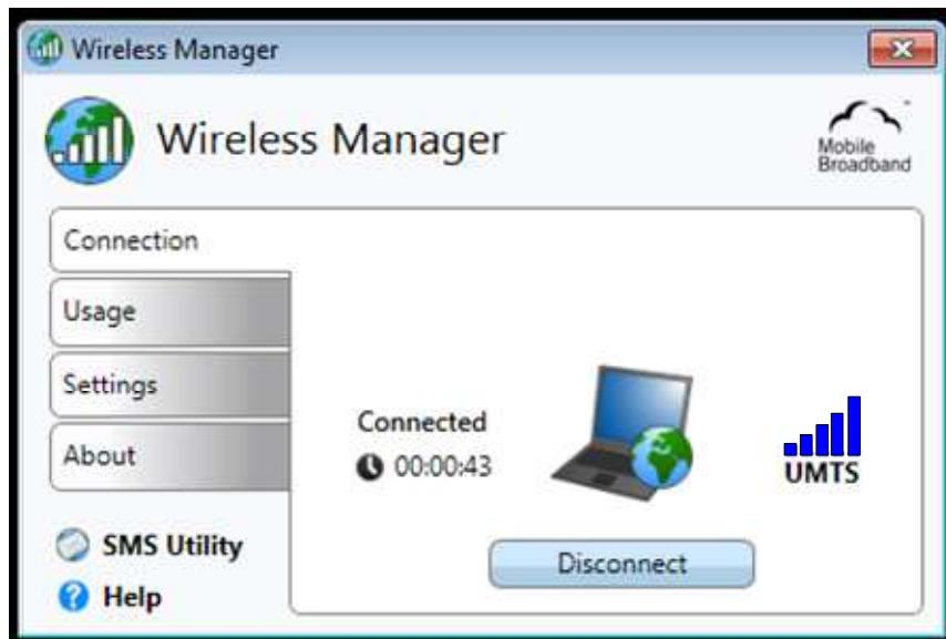
The network operator's and notebook manufacturer's logos can be customized in the application. Connection duration, connection mode, volume of data and an indication of the signal strength are provided in the Wireless Manager window while connection is active. The figures provide an approximate checkpoint of the data volumes. Please note that the information shown here is not guaranteed to match the mobile operator's bill.
