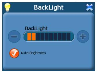
In the "Back Light" menu, if "Auto-Brightness" doesn't be chose, tap the left button to decrease the brightness gradually, tap the right button to increase the brightness gradually; if "Auto-Brightness" is chose, the brightness of the LCD will be adjusted as the surrounding brightness automatically, but the buttons aside the backlight is useless then.
