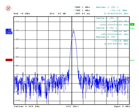
For band frequency 2.400GHz, test level is -79.12dBmW,
