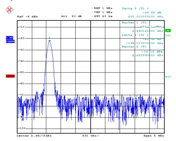
For band frequency 2.4835GHz, test level is -74.12dBmW,
