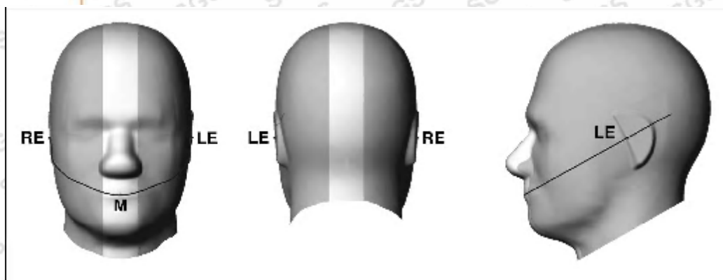
Figure 1—front, back, and side views of SAM (model for the phantom shell). Full-head model is for illustration purposes only—procedures in this recommended practice are intended primarily for the phantom setup of Figure 2. Note: The center strip including the nose region has a different thickness tolerance.
