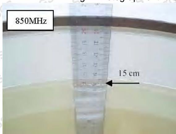
Fig.2 Photograph of the Tissue Simulant Liquid depth 15cm for Body Worn
